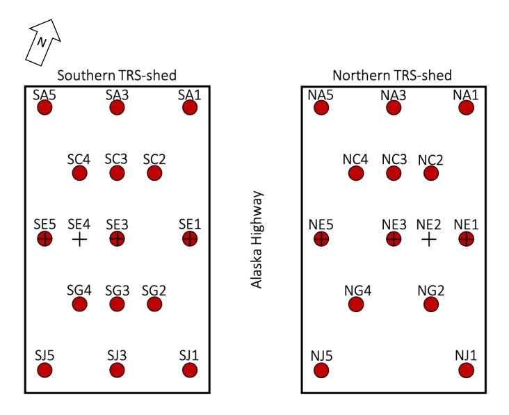
Location of the iButton sensors installed under the two sheds. The red circles represent sensors buried  $10\pm5$  cm belowground and the black crosses represent sensors attached to the roof with a rope and positioned 20 cm to 50 cm from the ground surface. The figure is not to scale.
